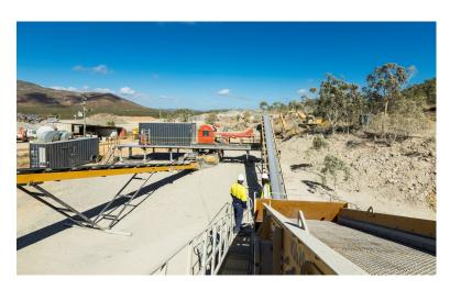
Figure 2 - XRT Sorter Pilot Plant
