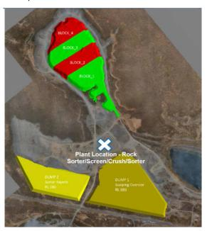
maximise its efficiencies to handle and process the material with minimal cost, producing a beneficiated XRT Sorter concentrate that can then be further processed through the Retreatment Plant on site.
