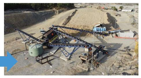
✓ Phase 1 Crushing and Screening Circuit Installed
