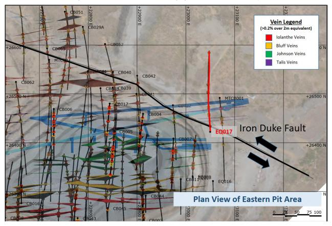
Fig. 4 - Plan View of Drill Hole EQ017 showing the Iron Duke Fault trace
