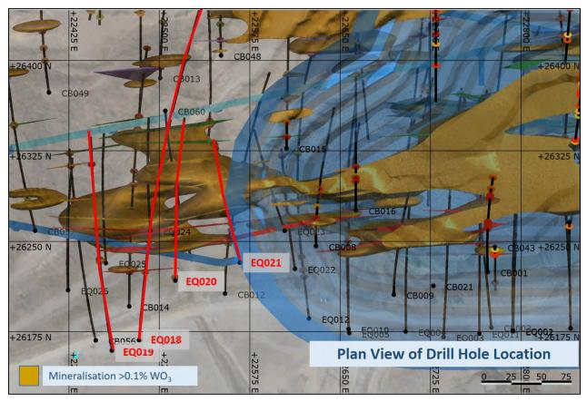
Fig. 3 - Plan View of Drill Hole Location (highlighted mineralisation >0.1 WO<sub>3</sub>)
