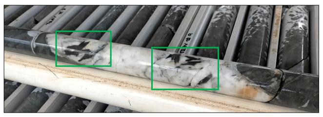
Fig. 1 - Black Wolframite Crystals (green frame) in a King-Vein in the West Dyke Area
