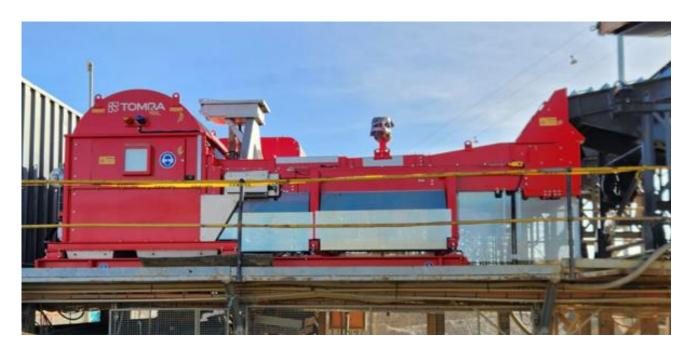
Fig.3 - Current XRT Sorter unit at Mt Carbine (two in operation, one under refurbishment)
