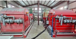
Fig.4 - Saloro's XRT Sorting Plant fully commissioned; 2x Tomra XRT Sorters (COM Tertiary XRT 1200)
