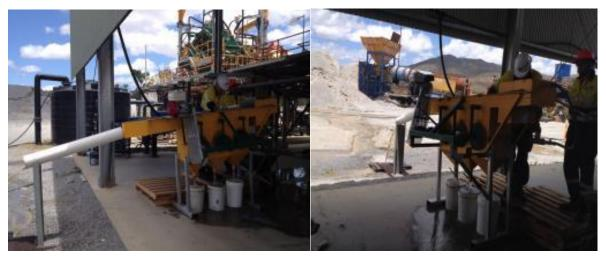
Jig test-work being carried out at the Tailings Retreatment operation.
