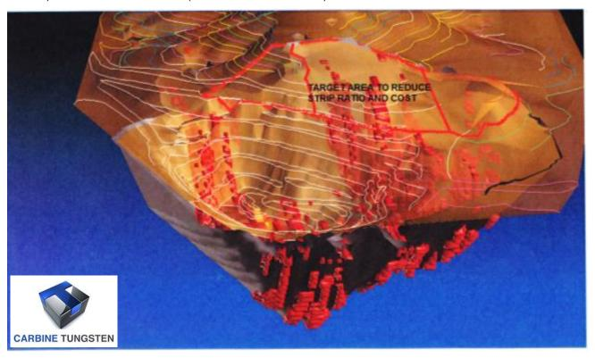
The above image is for the start of the open pit mining sequence of the Upper Ruby Zone benches of the existing pit.
