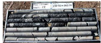
Interval assaying 3.69g/t Au from 138.5m to 140.65m in the dark grey/black carbonaceous fault gouge adjacent to altered monzodiorite in Icon drill hole ICK 002.
