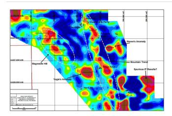
The above image shows IP chargeability at 100m below surface in part of Crow Mountain EL6648. The yellow (low) to dark red (high) represents chargeability implied to be due to the presence of conducting minerals in the subsurface. Sulphide mineral grains disseminated in listwanite may be causing the chargeability response.
