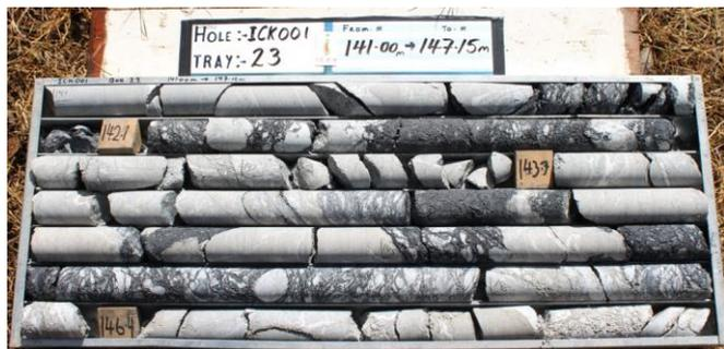
Interval assaying 8m at 1.27g/t Au from 140m in hole ICK001, showing carbonaceous gouge (dark grey) intruded by altered quartz monzodiorite dykes (light grey). It is now thought that most of the gold in this interval is in the carbonaceous gouge and this will be confirmed by further sampling.
