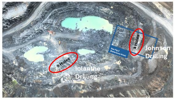
Fig.1 - Drone photo of pit after heavy rain when the veins are exposed; 13 RC holes drilled at 70 degress and 33m length each
