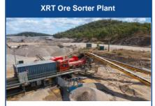
Sorter Feed undergoes 10x upgrade utilising X-Ray Technology and is transported to Gravity Beneficiation plant for tertiary crushing prior to gravity processing
