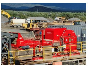
Fig.1 – 2<sup>nd</sup> TOMRA XRT Sorter (both XRT Sorters can operate in parallel or individually, utilising same product and waste conveyors)
