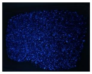
Medium -1mm + 0.3mm jig concentrate with UV light showing a large amount of scheelite.
