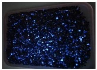
Coarse -3mm jig concentrate under UV light show that the scheelite is present as liberated grains.
