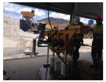
Jig Test Work – Tailings Retreatment Operation
