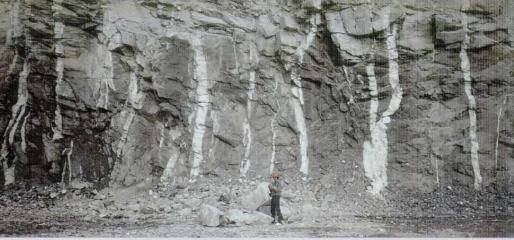
High Grade quartz-wolframite sheeted veining (open pit floor 1986)
