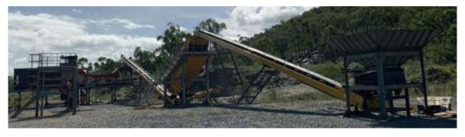
Figure 3: Sensor Based Sorting (XRT Pilot Plant)
