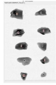
Typical X-Ray scan showing Tungsten Mineralization
