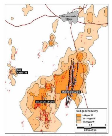
**Figure 4.2.** Plan showing Soil Geochemistry Data and Historical Workings of the Barruecopardo, Valdegallegos, Las Cabritas Tungsten Systems.
