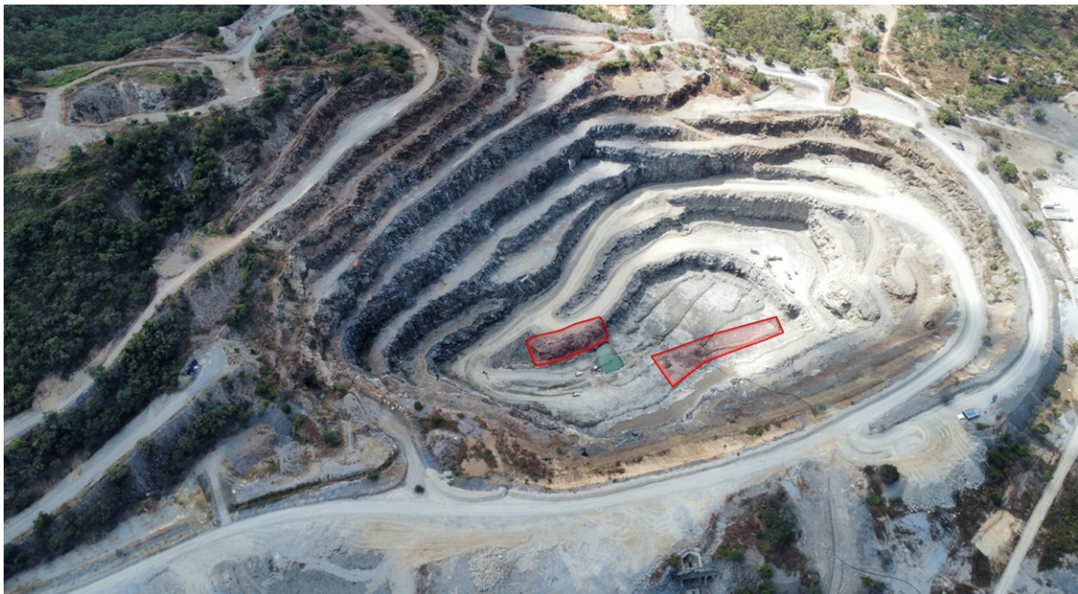
Fig. 4 - Dewatering of the Andy White open pit is complete and RC grade control drilling is underway. Red indicates the planned 1 st month of mining blocks.
