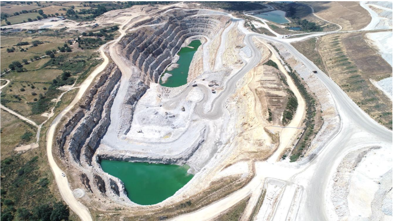
Figure 2: Lower Pit and Northern In-Pit Sump
