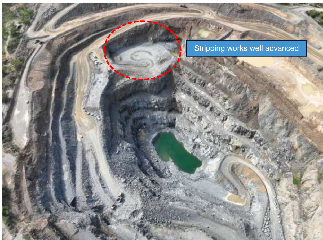
Pictured: Mt Carbine Mine January 2025 - Andy White Open Pit. The dotted line shows the new mine plan focus on waste removal to gain access to the high-grade Iolanthe ore reserves planned for the March 2025 quarter.
