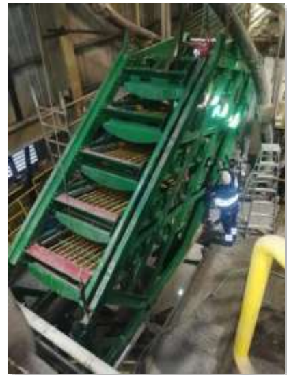
Pictured Left: Stockpile showing multi day feed buffer; Pictured Right: Multideck Screen underway for improved feed preparation in the Gravity Plant.
