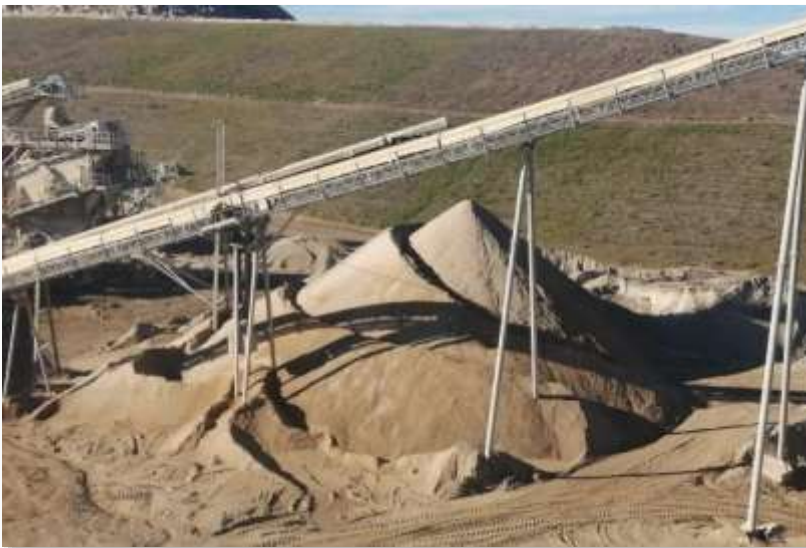
Pictured Left: Stockpile showing multi day feed buffer; Pictured Right: Multideck Screen underway for improved feed preparation in the Gravity Plant.
