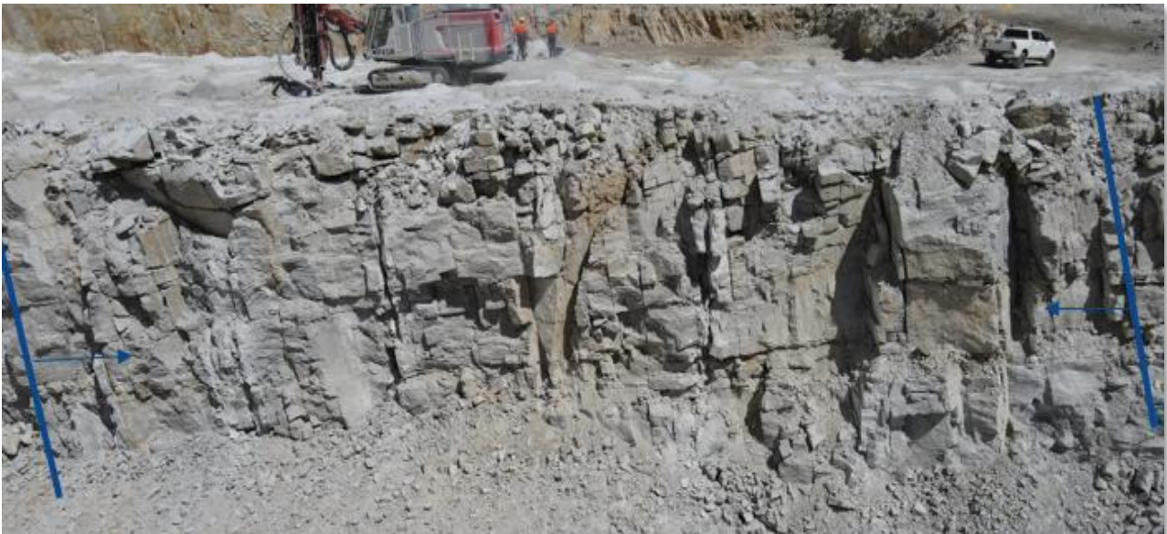
Pictured: A 10-metre bench face with the mineralised zones marked
