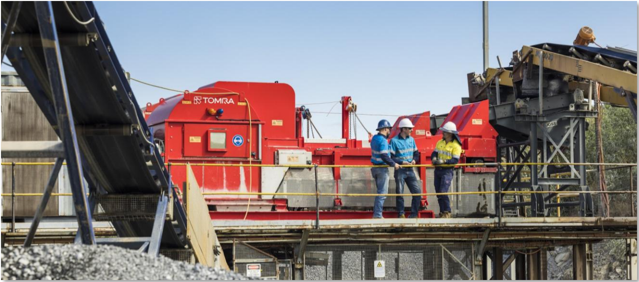
Pictured: XRT Ore Sorters at Mt Carbine: A key driver of efficiency and economic success, playing a crucial role in maximising the economic viability of operations by optimising ore processing, increasing feed grades, and reducing waste—ensuring sustainable and efficient production.
