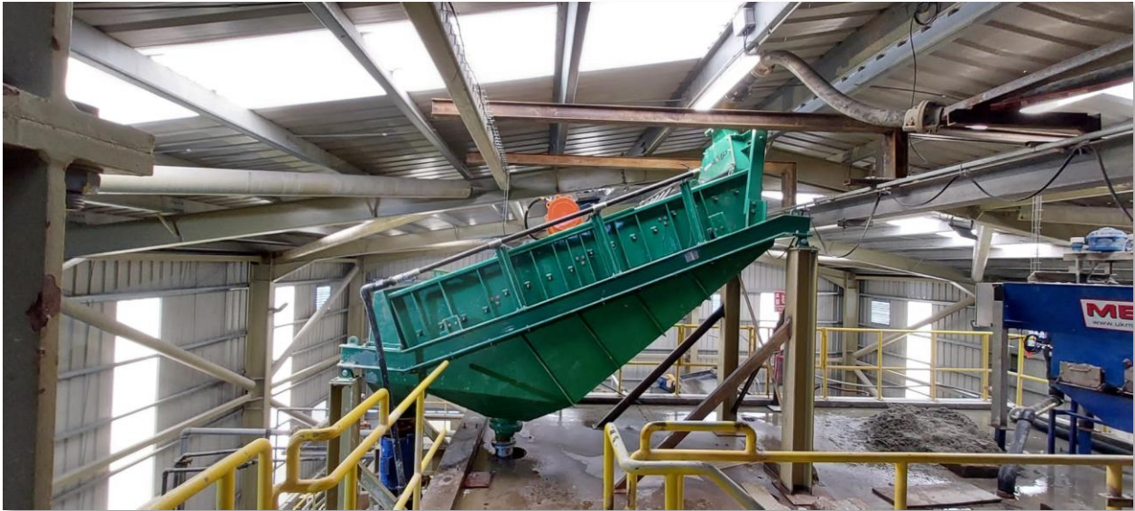
Pictured: The multideck screen being commissioned will optimise further the feed preparation to the Gravity Plant
