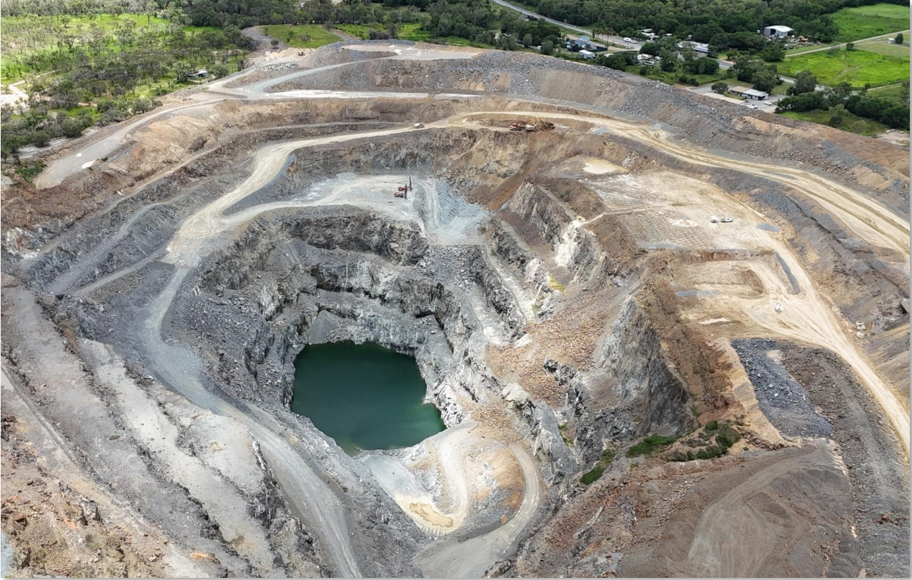
Pictured: The Andy White Open Pit at Mt Carbine end January 2025, mining operations entered the Stage II Open Pit and focused on stripping waste in cutback area.
