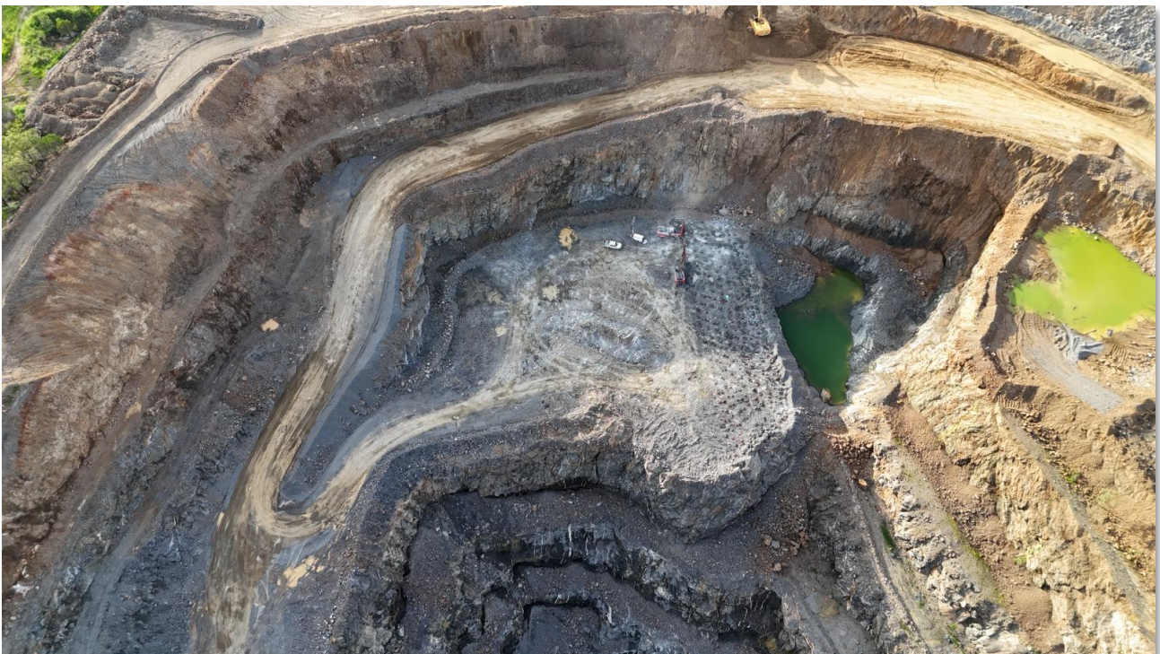
Pictured: The Southeast corner of the Open Pit, initial focus of the Stage II pit stripping and cut back with the Iolanthe and Bluff vein package as main targets with drilling progressing at 345-335 RL.
