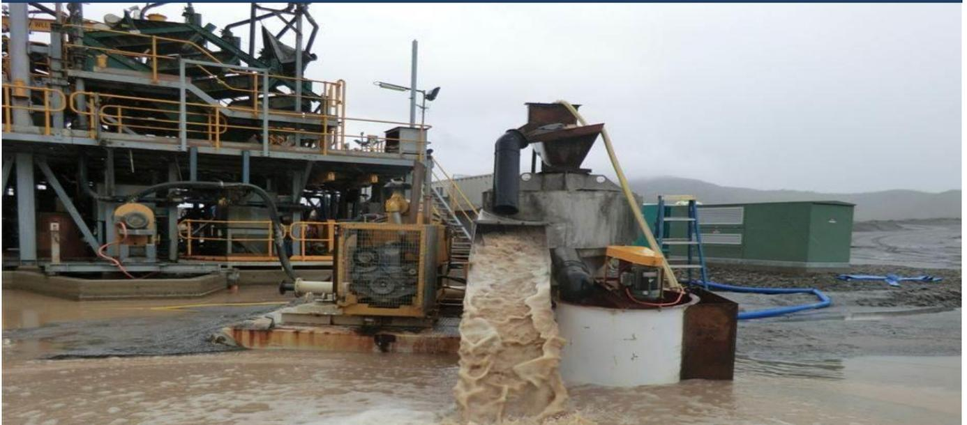
Testing of Ultra Fines Centrifuge recovering tungsten particles down to three micron
