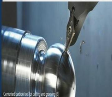
Cemented carbide tool for parting and grooving (3)
