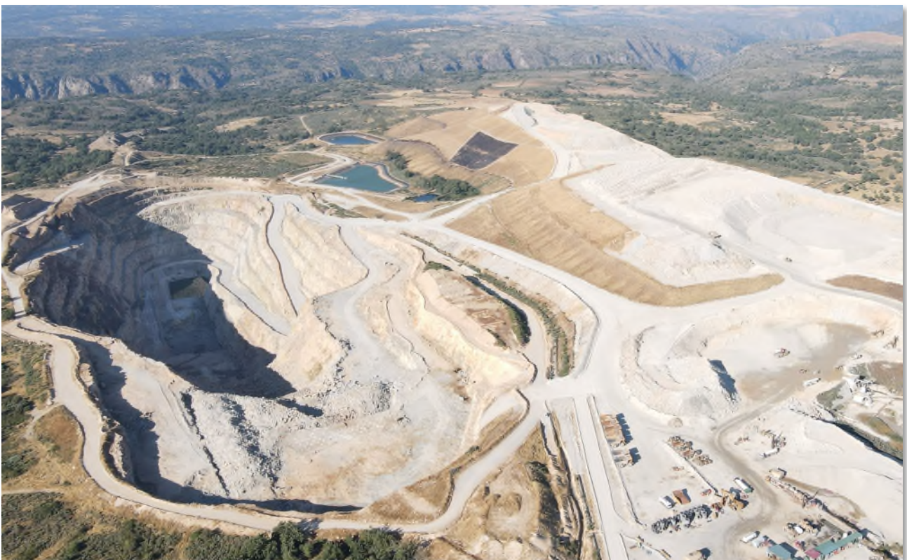
Picture above: Northern area of Phase 6 at elevation 700RL, including the access ramp and 690RL bench, with ore stockpile and waste dump as of the end of June 2025.
