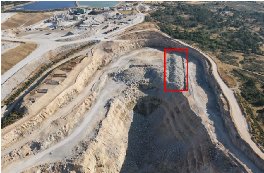
Picture above: The Northern Area of the Open Pit. Red rectangle shows two blasts containing Ore waiting to be hauled to the feed stockpile. June 2025.
