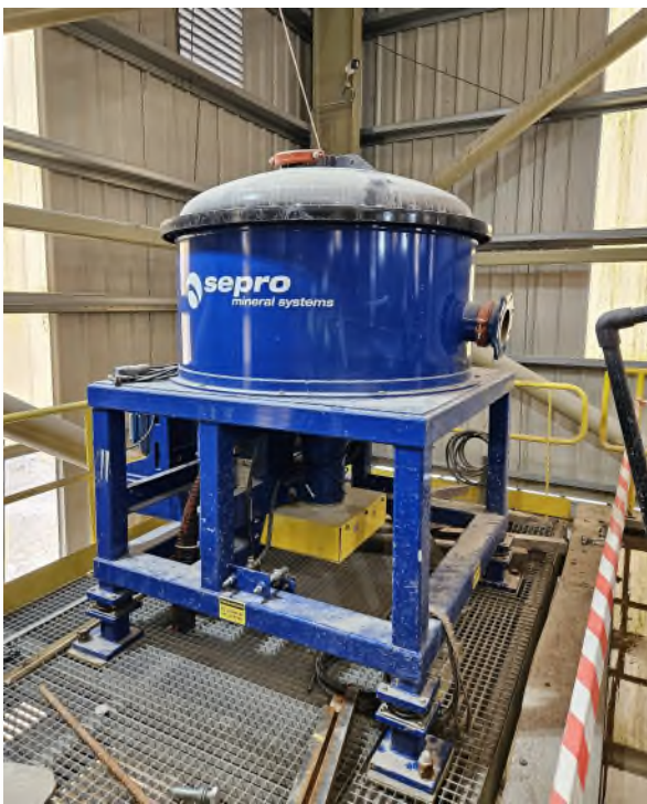
Picture above: The Falcon Concentrator before commissioning in the Processing Plant
