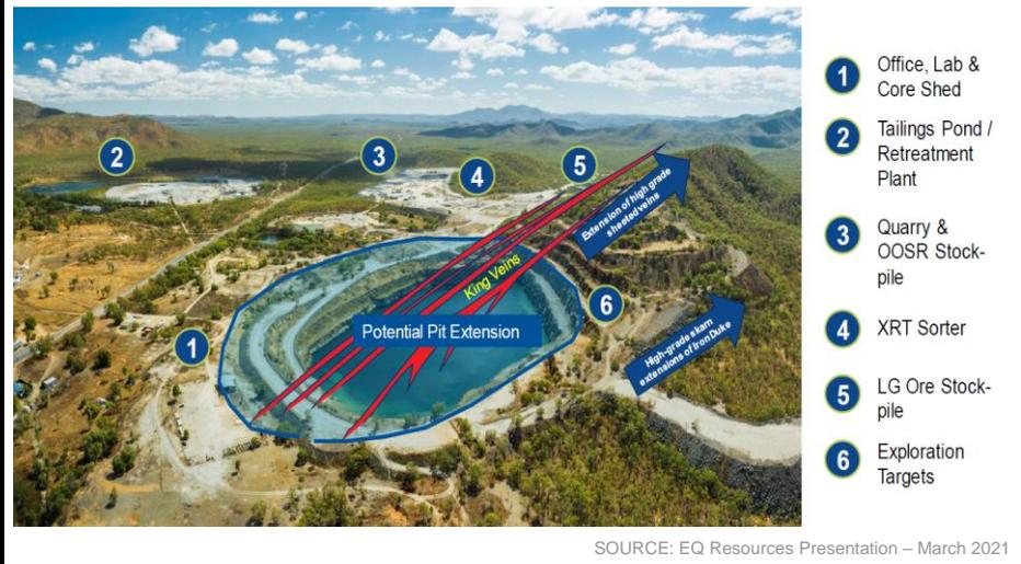
The Petersen's lodes are 2km southeast from the Mt Carbine open pit. Historic production at a grade of 0.6%  $WO_3$  resulted in production of 950t – 95,000 MTU – of scheelite concentrate. The mineralised zone is approximately 10m wide, and extends 1.3km along strike at surface.
