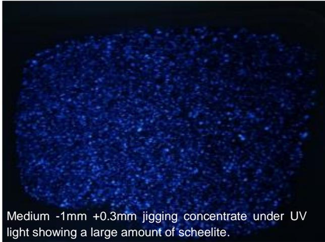
Medium -1mm +0.3mm jigging concentrate under UV light showing a large amount of scheelite.
