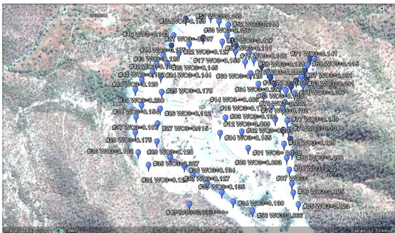
Figure 2. Aerial view of low grade stockpile showing locations of grab samples taken for characterisation of mineralogy and chemistry of stockpile for environmental permitting purposes. Each grab sample was approximately 20kg.
