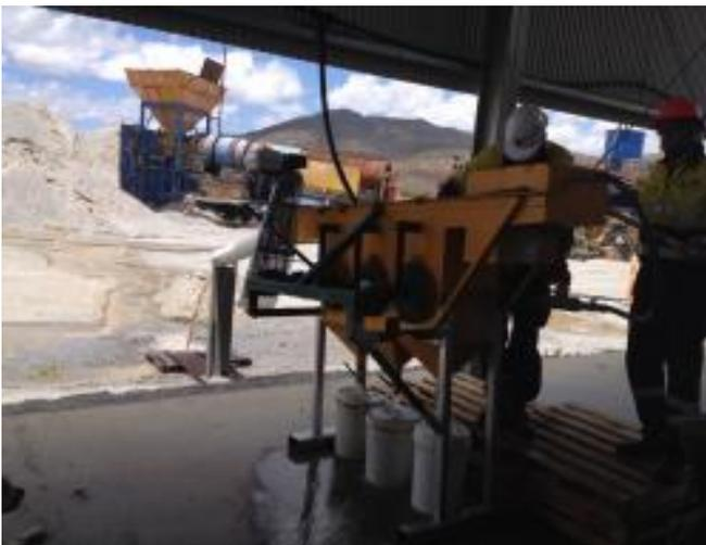
Jig Test Work – Tailings Retreatment Operation
