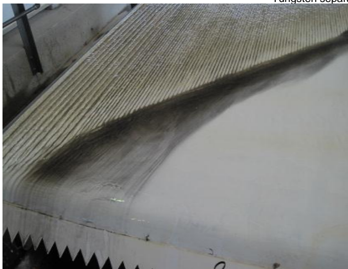
Tungsten separation on shaker tables
