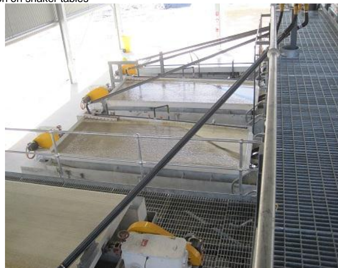
Tungsten separation on shaker tables
