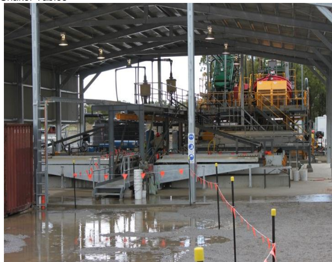
Tungsten separation on shaker tables
