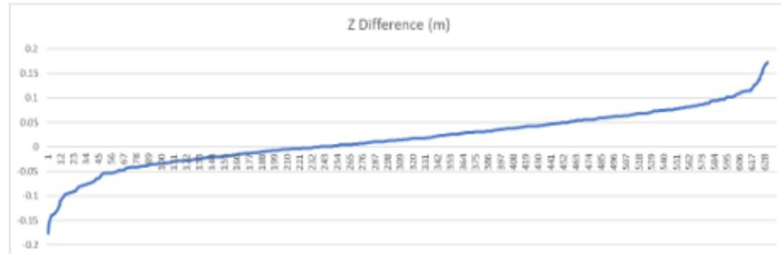
The above figures have been derived by comparing independently observed RTK GPS points against the resulting 3D photogrammetry model.
