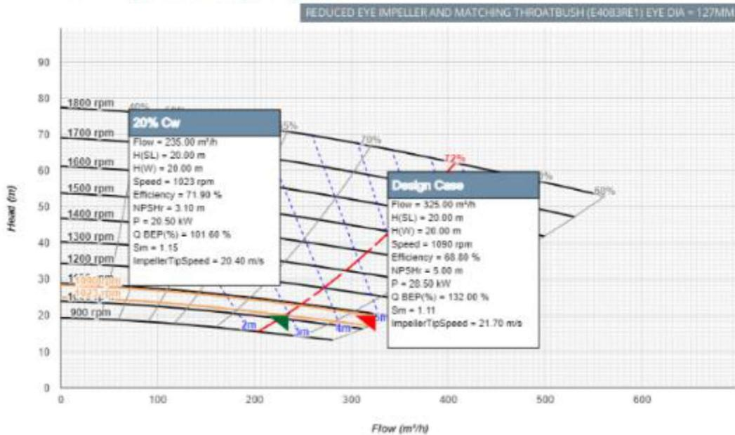
Figure 35: Assumed Operation of PU-024A with 6/4AH
