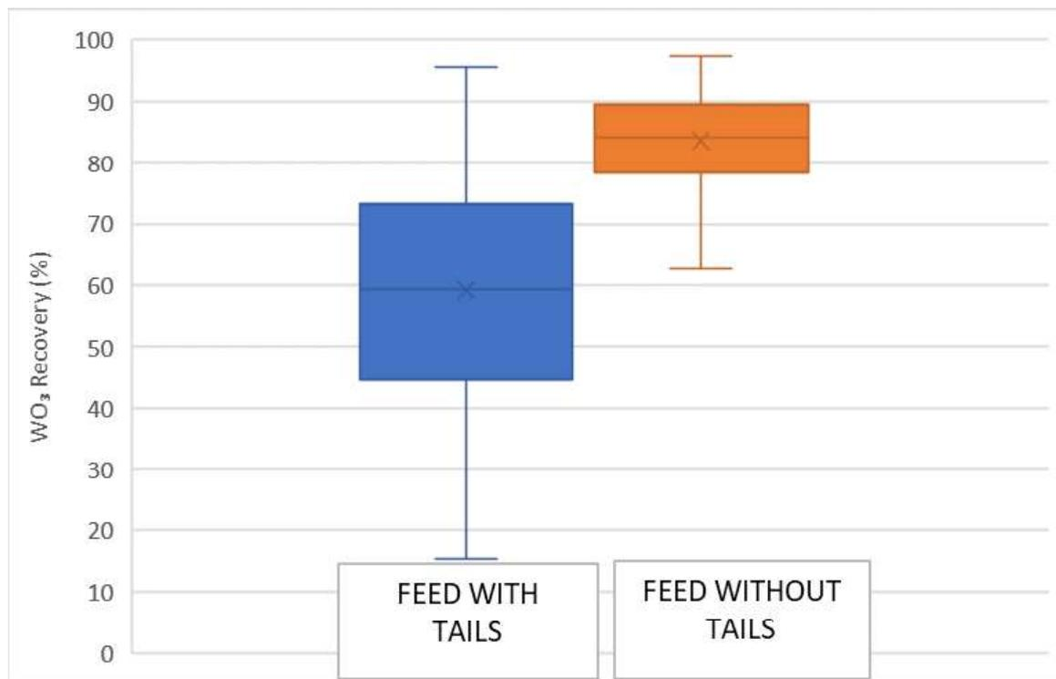
Figure 45: Plant Recovery Comparison with Tails and without Tails
