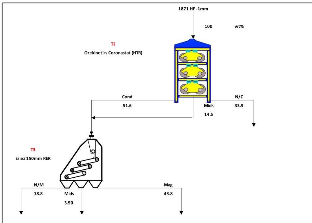
Figure 51: Combined Electrostatic and Magnetic Separation Test Flowsheet
