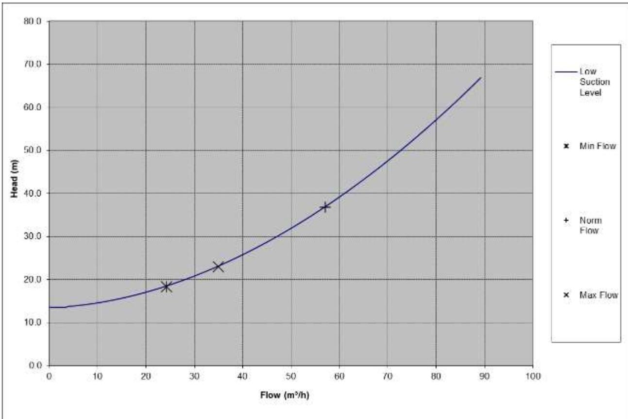
Figure 31: System Curve for PU-008
