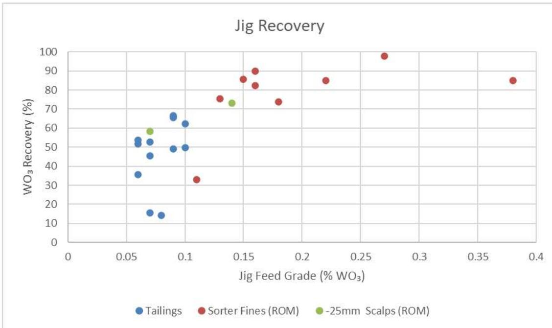
Figure 43: Jig Recovery vs Feed Grade by Feed Type
