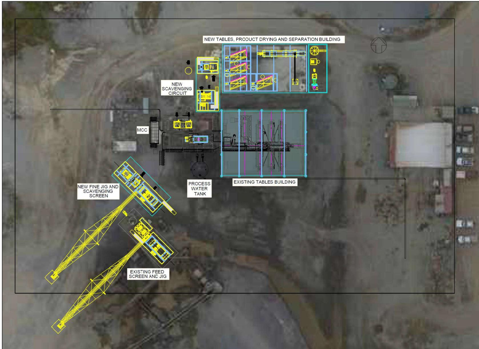
Figure 55: Process Plant Site Layout
