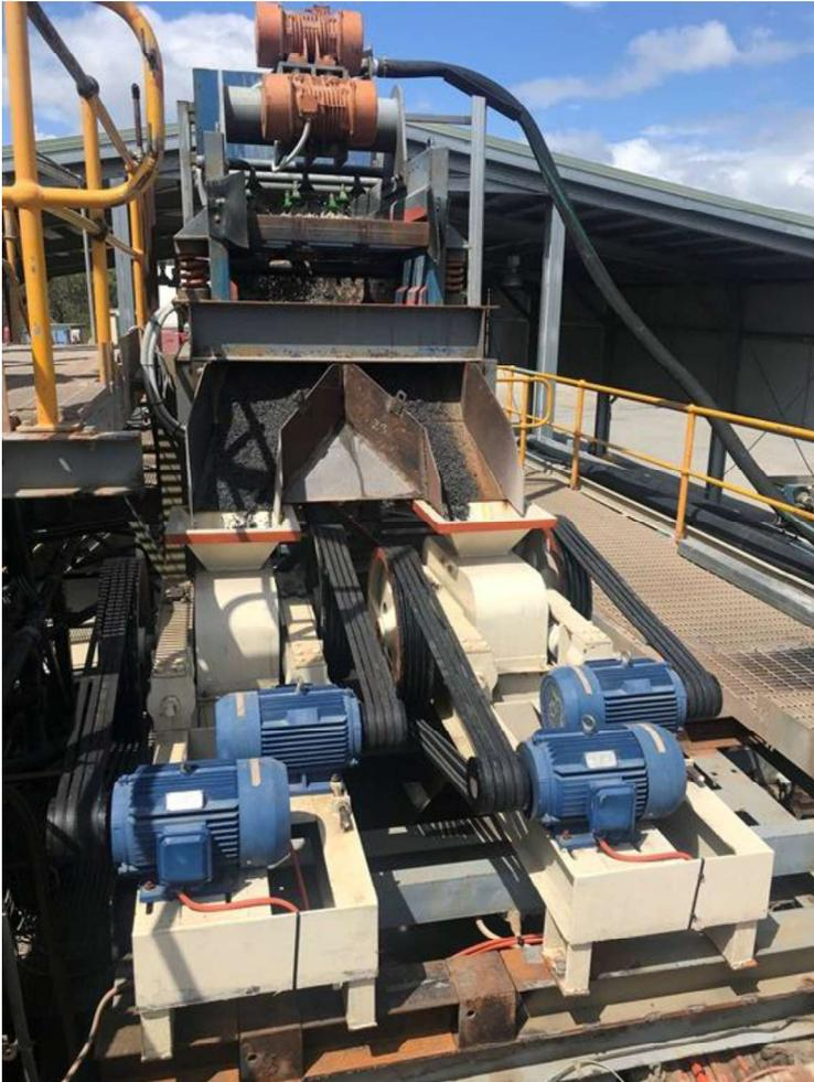
Figure 39: Screen and Rolls Crusher
