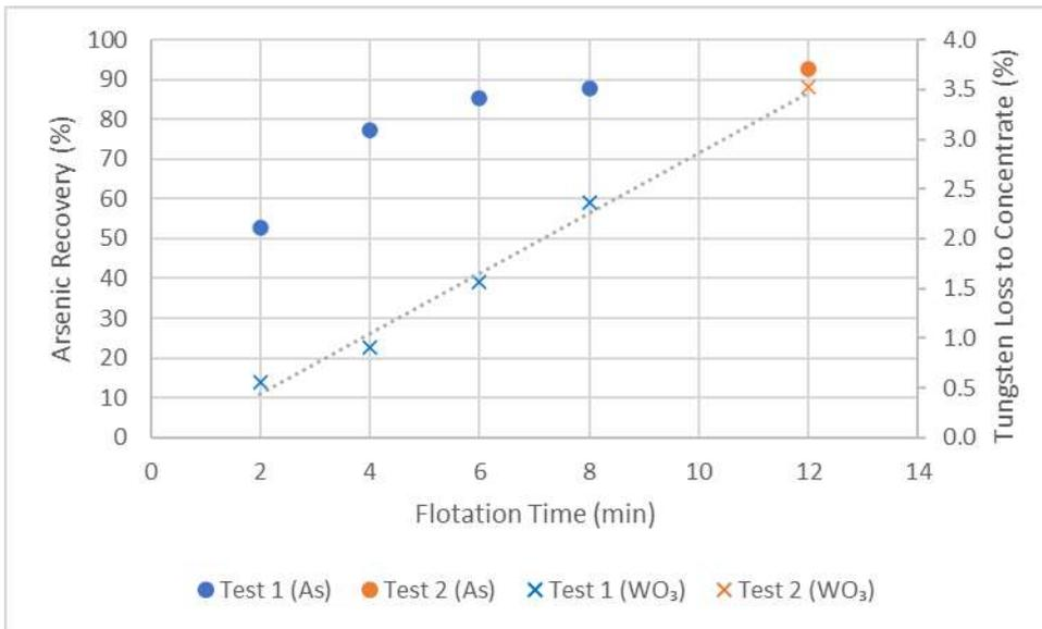
Figure 48: Arsenic and Tungsten Recovery for Test 1 (75 µm) and Test 2 (100 µm)
