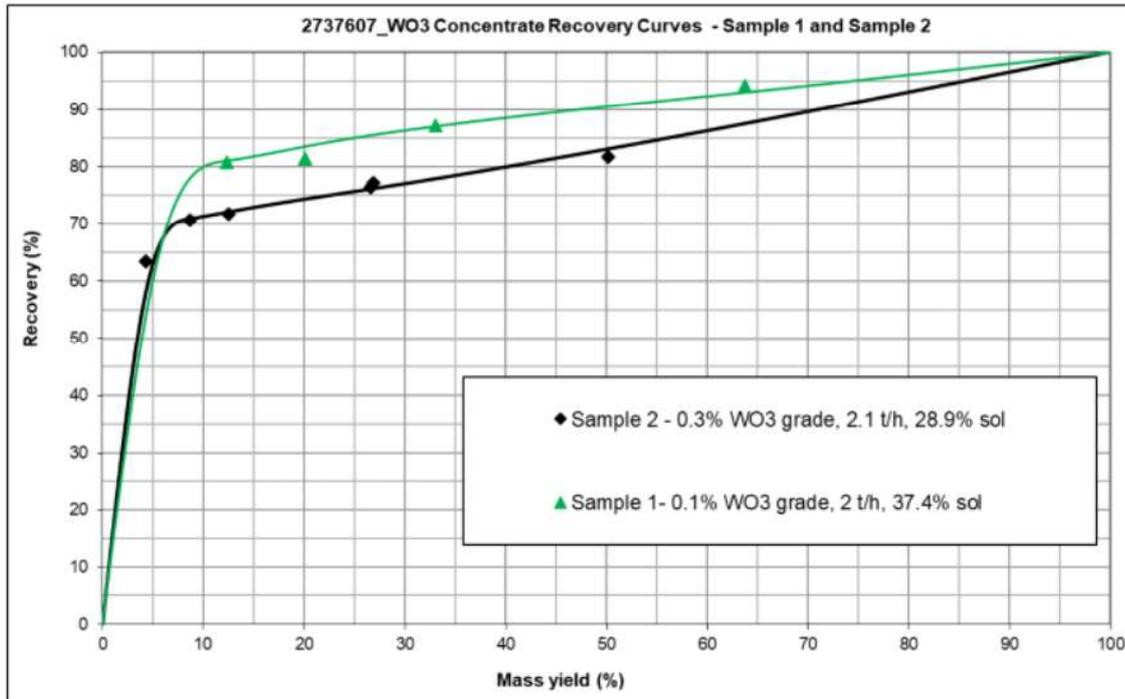
Figure 46: Mass vs Tungsten Recovery for Coarse Tailings (Sample 1) and Low Grade Fines (Sample 2)
