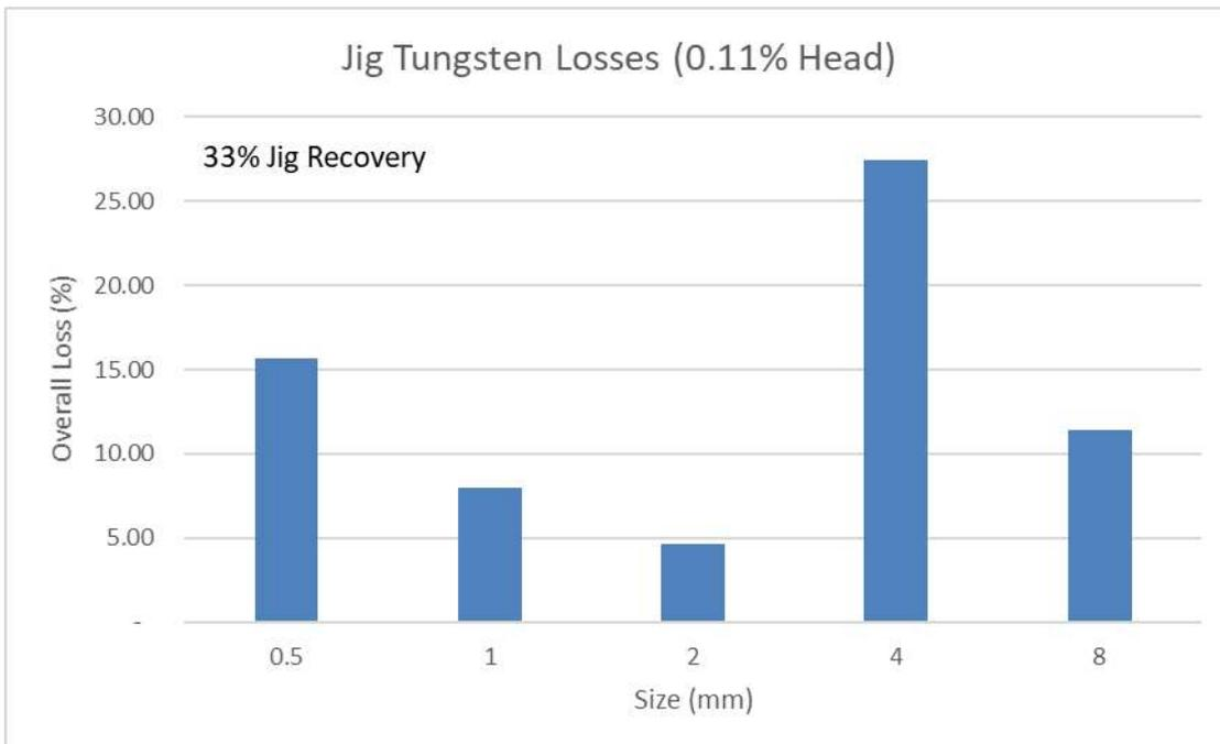
Figure 44: Jig Losses by Size for a Low Tungsten Tailings Feed
