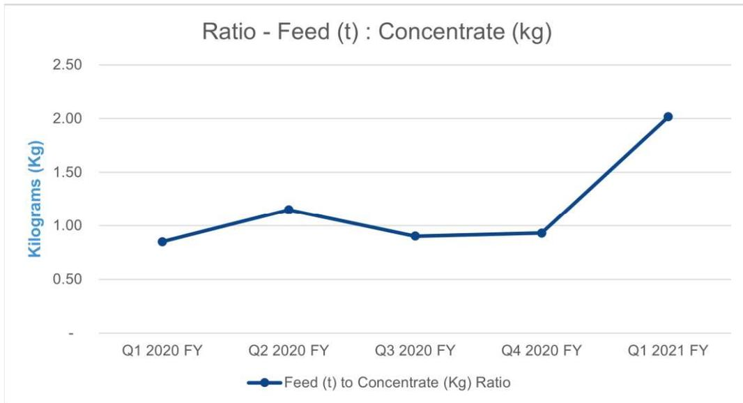
Figure 27: Ratio of concentrate produced from feed processed
