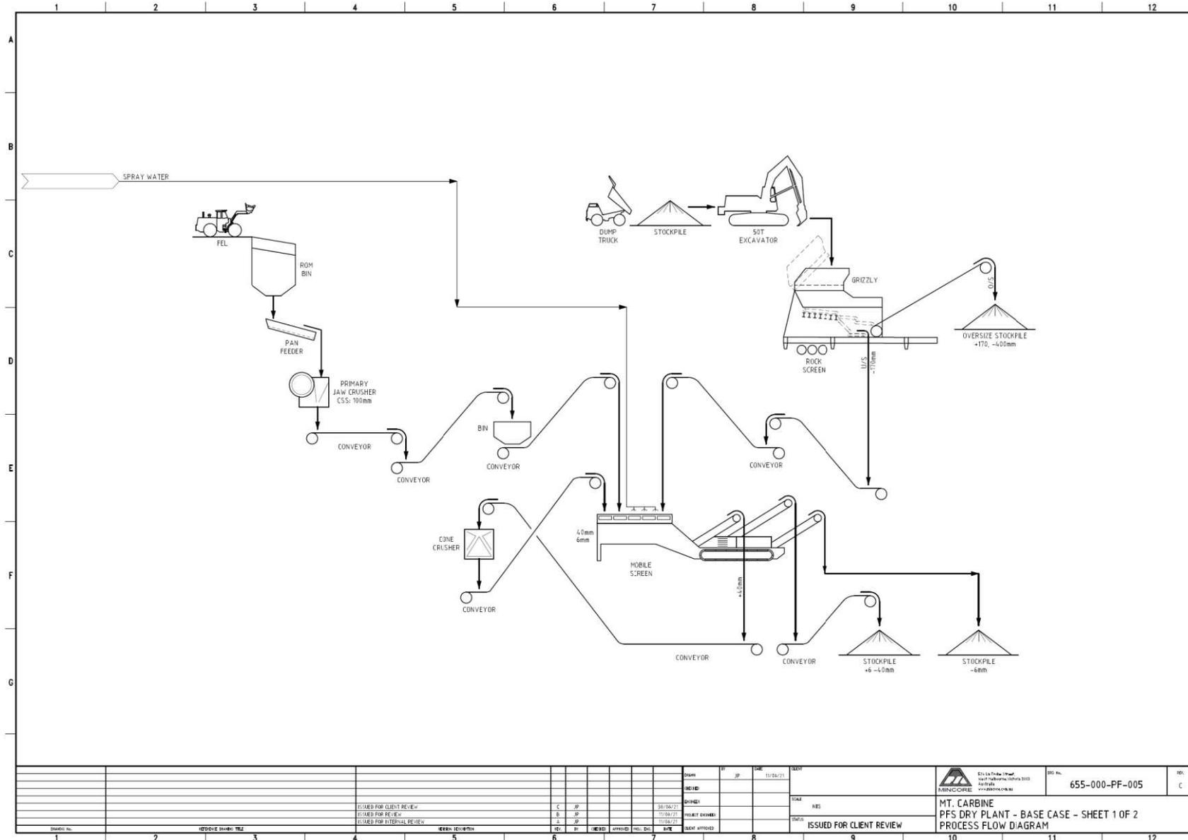
Figure 4: Existing Crushing and Screening Process Flowsheet
