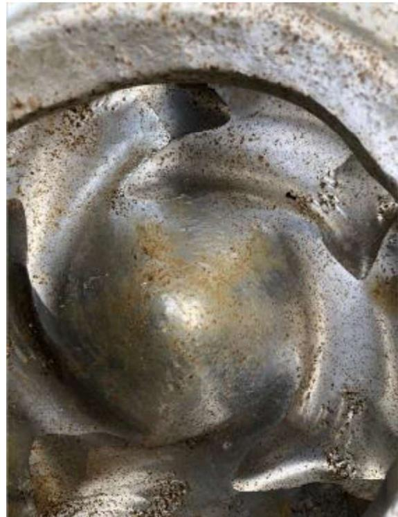
Figure 36: AH 4/3 Impellor Wear
