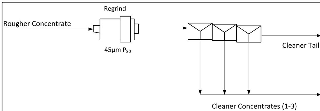
Figure 49: Cleaner Flotation Test Flowsheet
