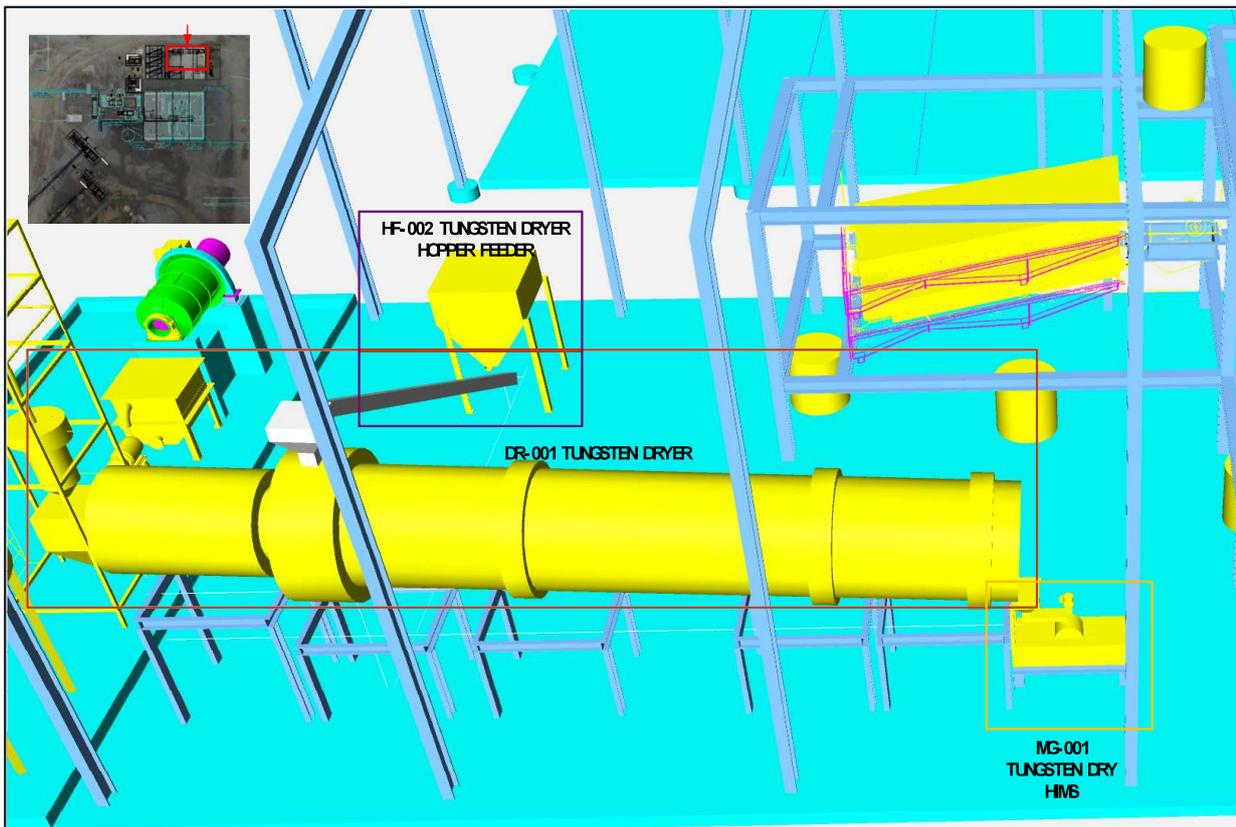
Figure 61: Tungsten Drying and Product Separation
