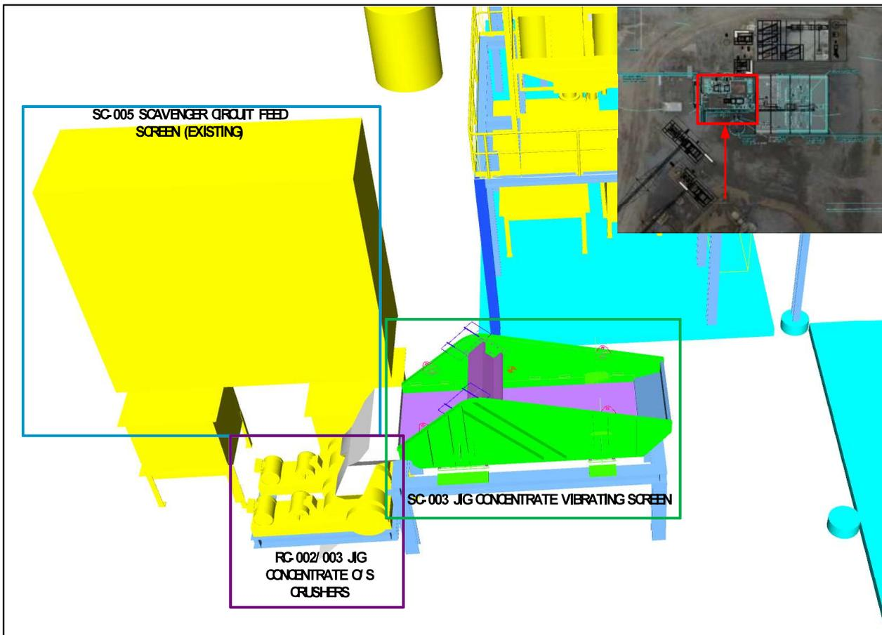
Figure 58: Upgrade Jig Concentrate Screen and Jig Oversize Crushing
