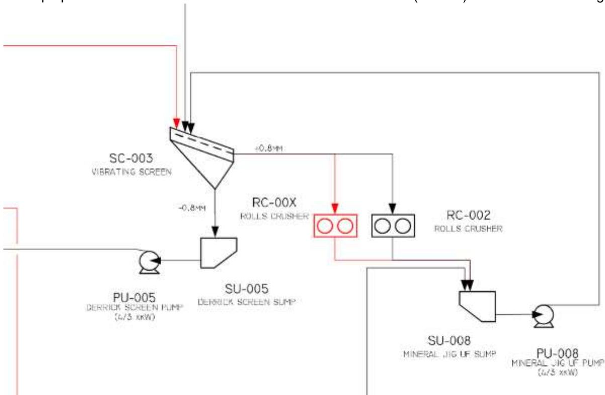
Figure 40: Additional Rolls Crusher in Flowsheet
