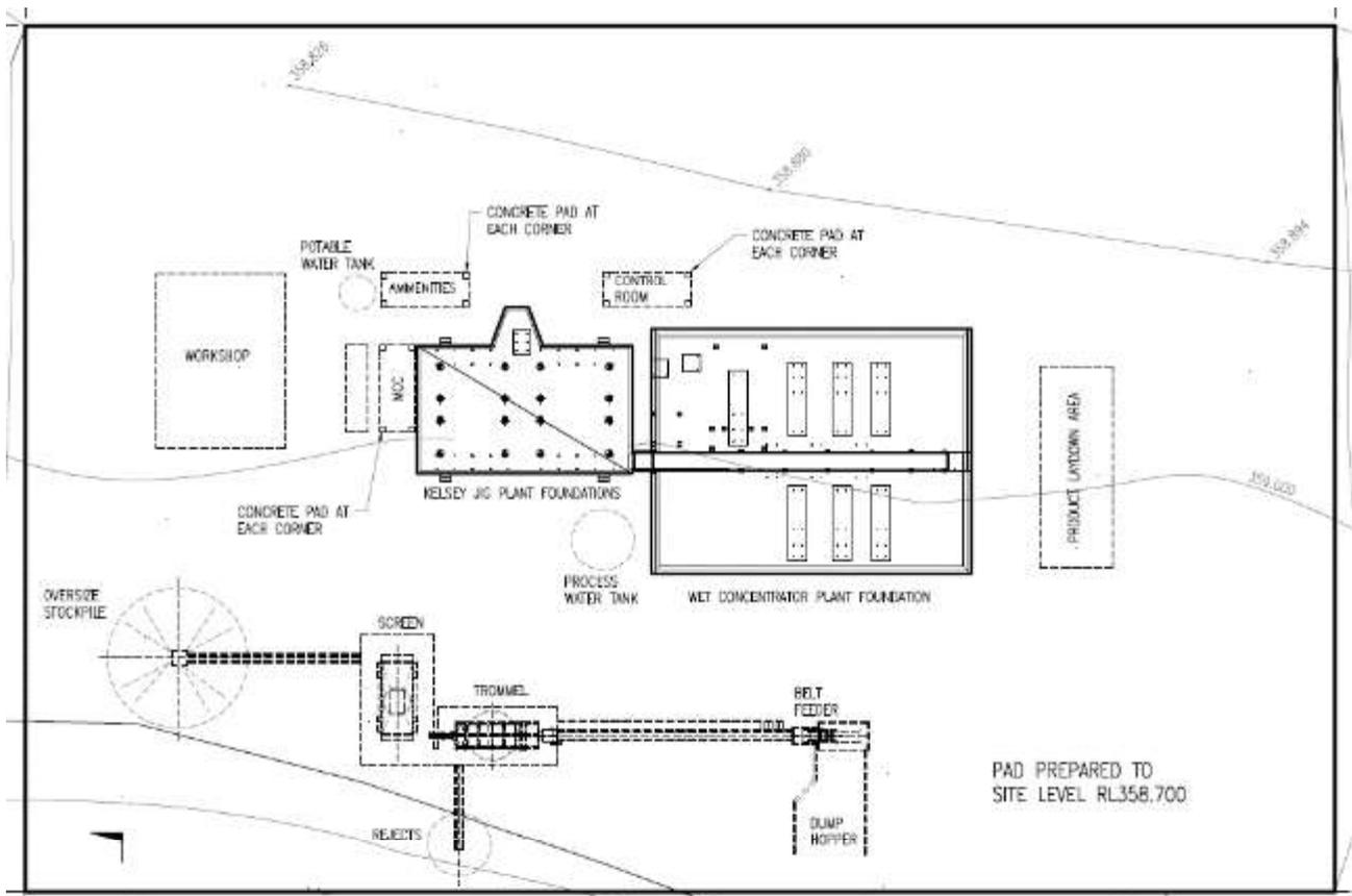
Figure 25: Gravity Processing Plant Site Layout
