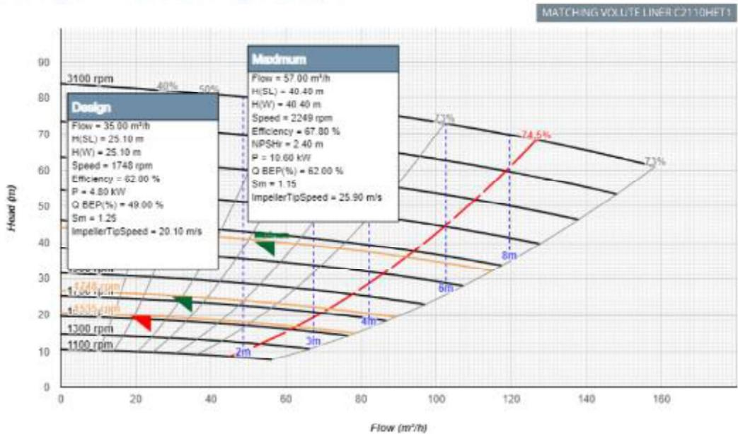
Figure 33: Curve for Smaller Pump in the PU-008 duty (3/2AH)
