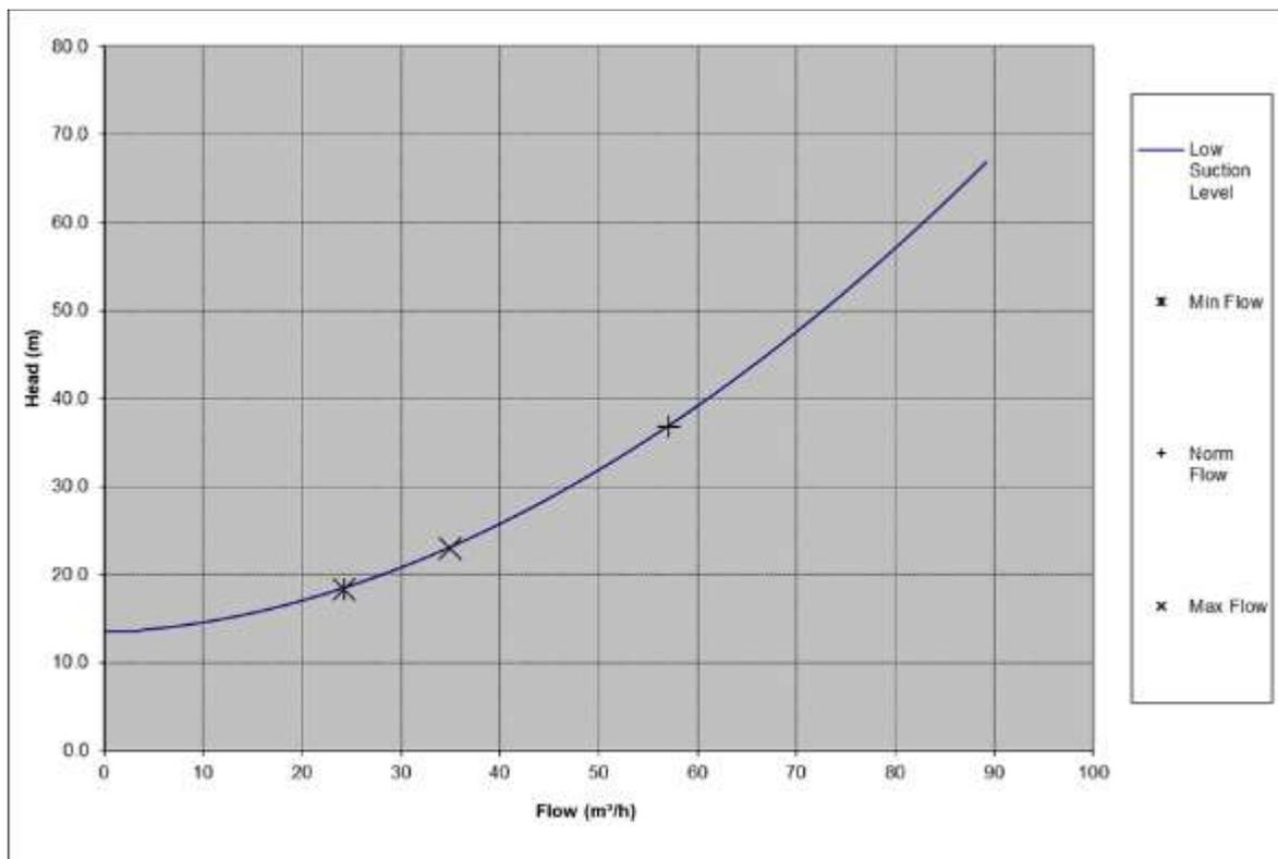
Figure 34: System Curve for PU-024A
