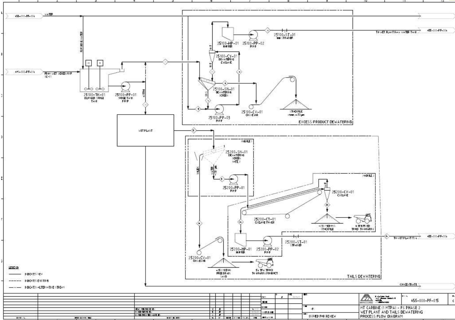
Figure 22: Excess Product Dewatering and Tailings Dewatering
