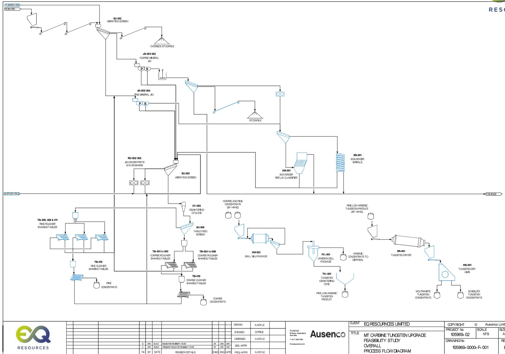
Figure 53: Overall Circuit Block Flow Diagram
