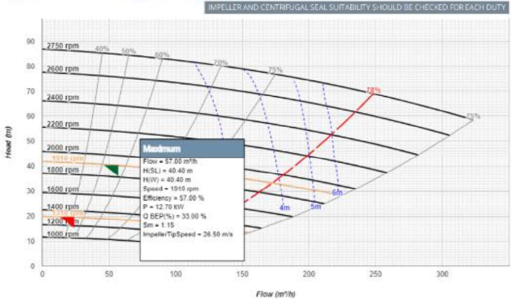
Figure 32: Assumed Operation of PU-008 with 4/3AH
