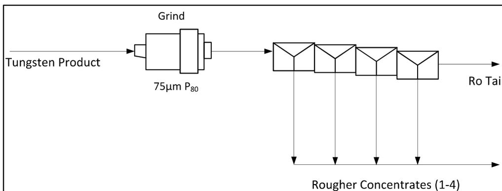
Figure 47: Rougher Flotation Test Flowsheet
