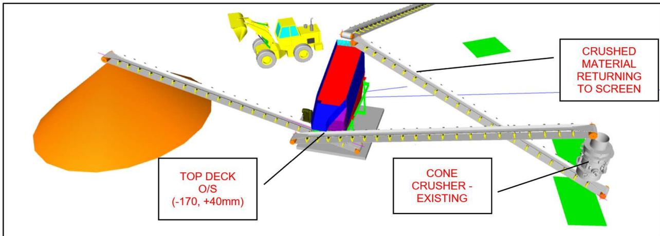
Figure 10: Cone Crushing Circuit
