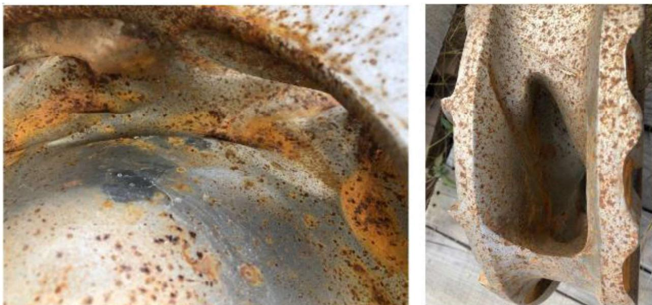
Figure 38: AH 6/4 Impellor Wear Photos
