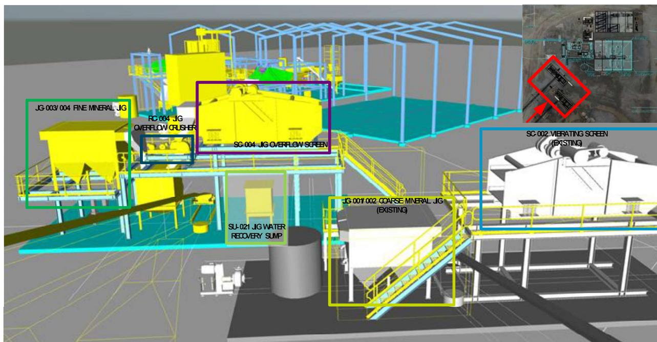
Figure 56: Fine Mineral Jig, Overflow Screen and Crushing Plant
