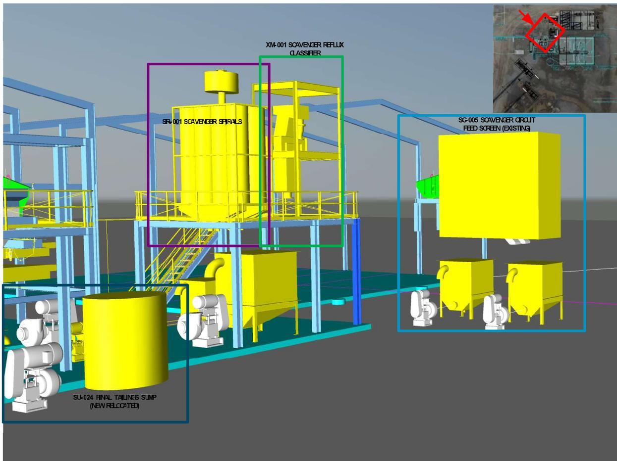
Figure 57: Jig Overflow Scavenging Area
