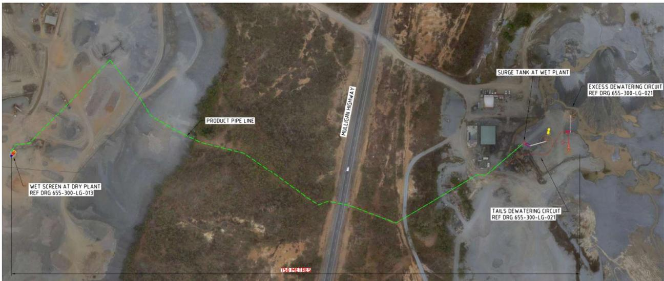
Figure 15: Product Transfer Pipeline Route
