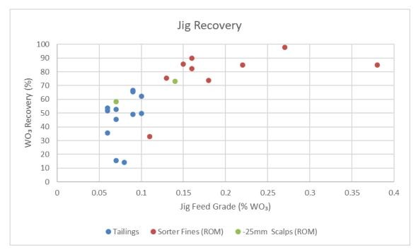
Figure 20: Jig Recovery vs Feed Grade by Feed Type
