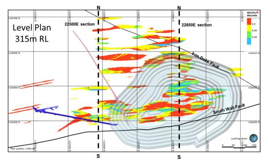
Figure 10: Plan of Block Model showing Tungsten Grade with Pit Overlay
