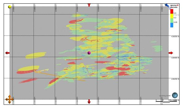
Figure 9: Plan of Block Model showing Tungsten Grades (WO3 %) for entire resource
