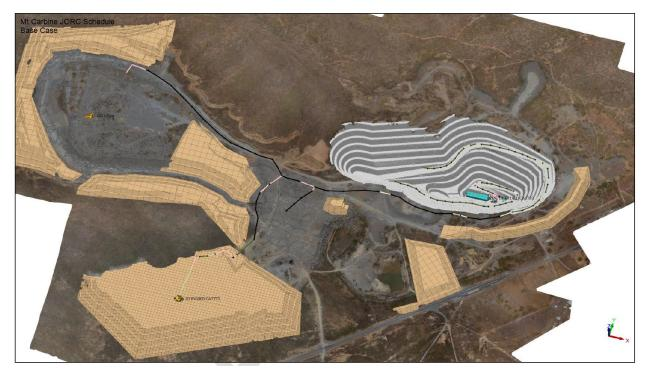
Figure 13: Isometric View of Ore Reserves Pit Shell
