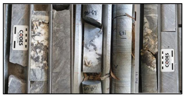
Figure 3: King Veins Showing Coarse Vein Textures of Wolframite Crystals
