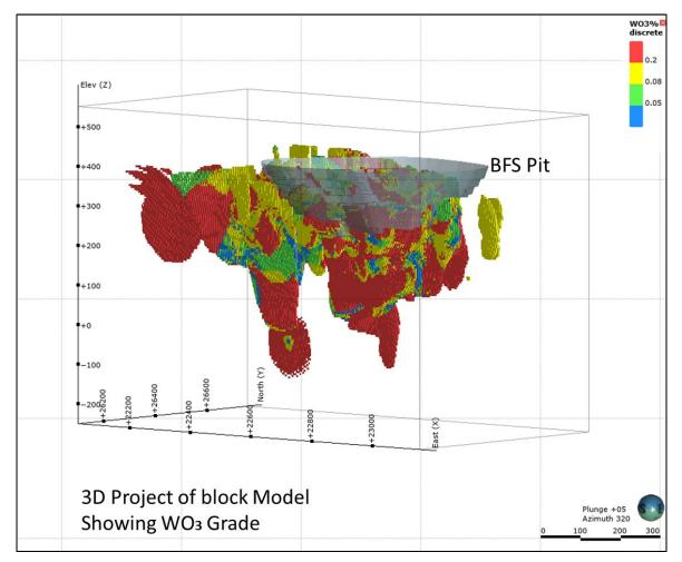
Figure 7: 3D perspective view of the block model showing tungsten (WO<sub>3</sub>) grades
