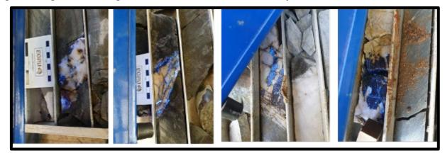
Figure 4: Core Showing Late Replacement of Wolframite by Fine Network Retrograde Scheelite
