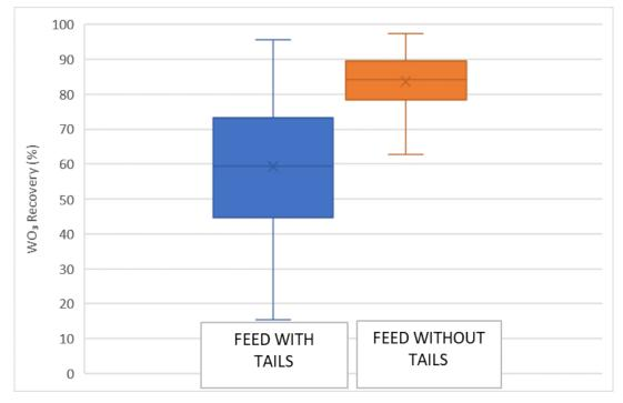
Figure 21: Plant Recovery Comparison with Tails and without Tails
