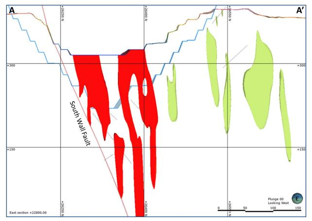
Figure 6: Typical Ore Section Through Open Pit
